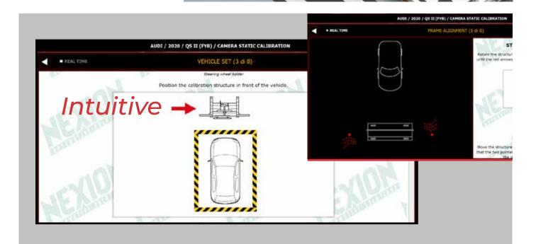
Intuitive. Error-proof. The software contains the preloaded positioning values. It displays the current position and guides the system in carrying out the operations (patented).
