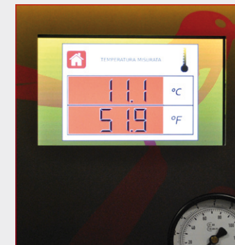
<15 and >30°C, red = do not work on tyre
