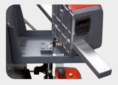
1 CCD sensor heads available in wireless or cable versions. Wireless version on 2.4 GHz industrial radio frequency. Battery charging on cabinet. The battery charger can support both the sensor heads and the clamps.
