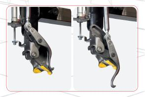
HEAD UNIT The demounting procedure uses the same working movements but absolutely no effort is required from the operator thanks to the "Leva Ia Ieva" (Without Iever) technology incorporated in the head (Patent Pending).
