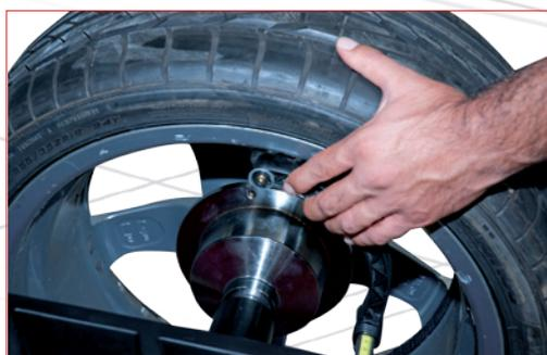
With automatic internal measurement sensor for measuring wheel distance and diameter. May also be equipped with EG1 electronic width sensor. Also available as version with manual internal measurement.
