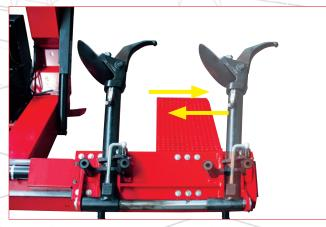
Carriage with hydraulic left-right translation and tool arm with safety lock system.
