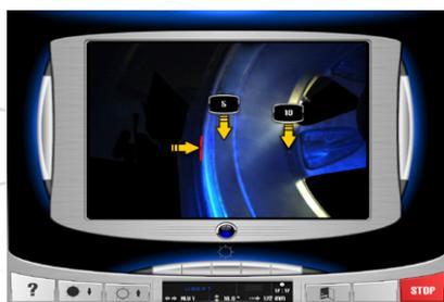
Professional quality video camera and advanced Corghi patented artificial vision technology to acquire and process the wheel image, and identify the balancing planes.
