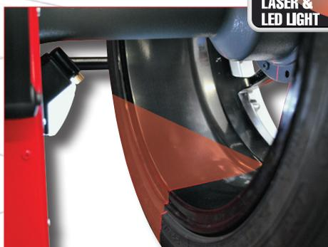
**LED spotlight** to light-up the work area and make it easier to clean the rim, check the wheel and apply weights. The adhesive weights can be positioned extremely rapidly using the laser pointer at 6 o'clock.
