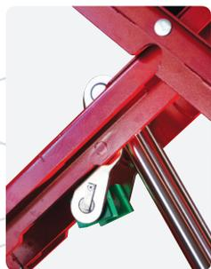
Special initial lift assist linkage for lifting loads even at minimum runway height.
