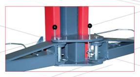
· Arm attachment trolley unit, compact and with reduced overall dimensions from the ground.
