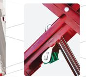
Special initial lift assist linkage for lifting loads even at minimum runway height.
