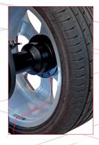
Three modes to position the adhesive weights: with the weight holfer clip (optional), with the 6 o'clock laser indicator (optional) or manually at 12 o'clock.
