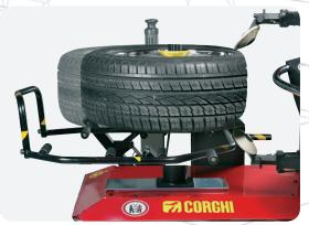
The **mounting/demounting tools** and bead breaker disk positioning is electronically managed by the machine according to the rim diameter, so as to ensure optimal working distances in any situation.
